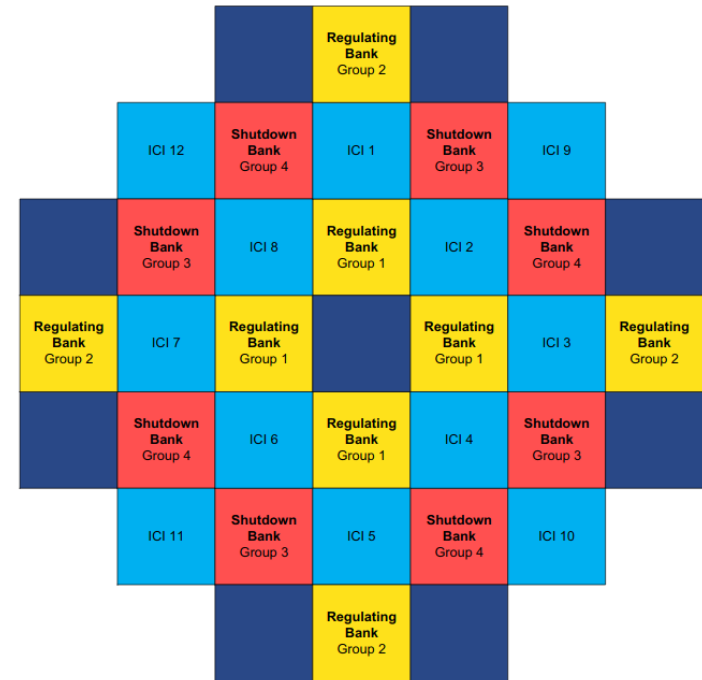
Figure 4.3-18: Control Rod and Incore Instrument Locations
